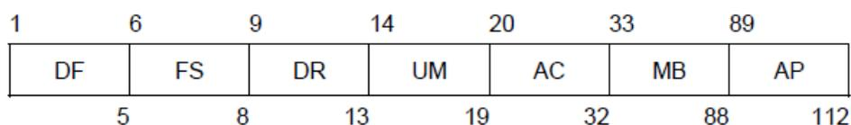
This reply shall be generated in response to an interrogation UF 4 or 20 with an RR field value greater than 15. The format of this reply shall consist of these fields:
