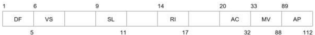
This reply shall be sent in response to an interrogation with UF equals 0 and RL equals 1. The format of this reply shall consist of these fields:
