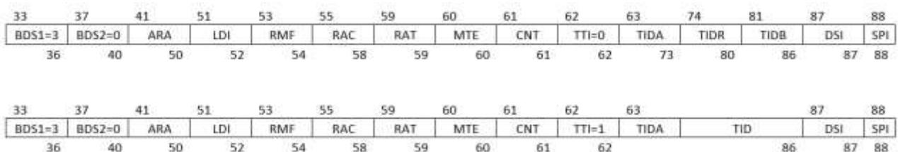
4.3.8.4.2.2.3 Subfields in MB for the data link capability report. When BDS1 = 1 and BDS2 = 0, the following bit patterns shall be provided to the transponder for its data link capability report:
