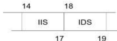
The following subfields shall be inserted by the transponder into the UM field of the reply if a surveillance or Comm-A interrogation (UF equals 4, 5, 20, 21) contains DI = 1 and RSS other than 0:
