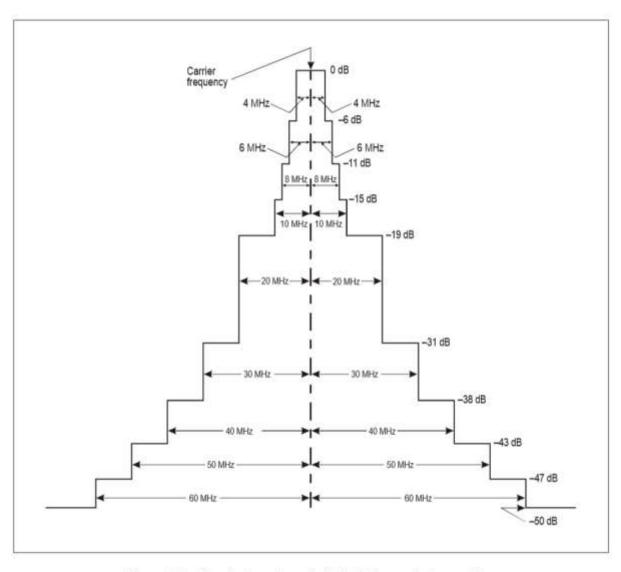
Figure 3-2. Required spectrum limits for interrogator transmitter
