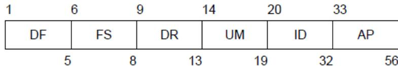
This reply shall be generated in response to an interrogation UF 5 or 21 with an RR field value less than 16. The format of this reply shall consist of these fields:
