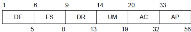
This reply shall be generated in response to an interrogation UF 4 or 20 with an RR field value less than 16. The format of this reply shall consist of these fields:
