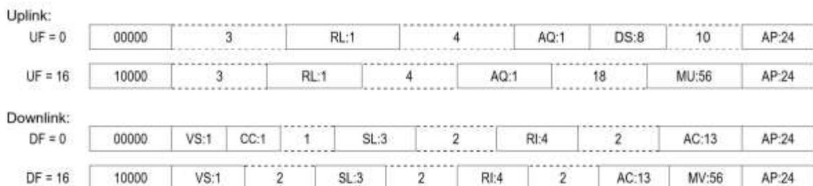
Figure 4-1. Surveillance and communication formats used by ACAS
