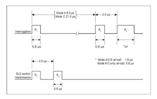
Figure 3-3. Intermode interrogation pulse sequence
