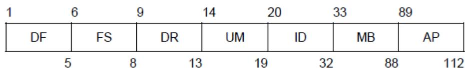
This reply shall be generated in response to an interrogation UF 5 or 21 with an RR field value greater than 15. The format of this reply shall consist of these fields:
