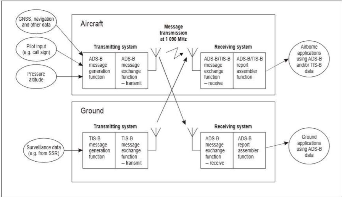
Figure 5-1. ADS-B/TIS-B system functional model
