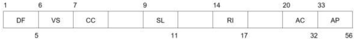
This reply shall be sent in response to an interrogation with UF equals 0 and RL equals 0. The format of this reply shall consist of these fields:
