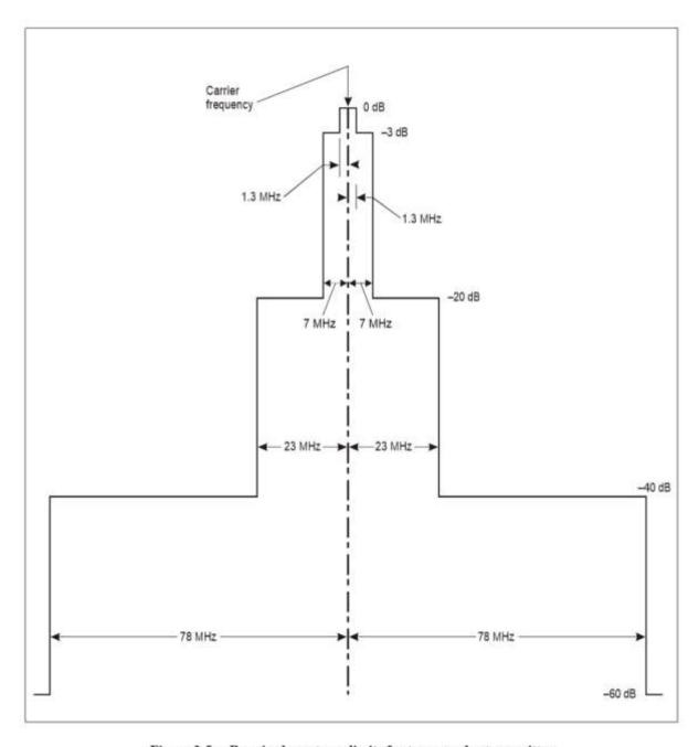
Figure 3-5. Required spectrum limits for transponder transmitter
