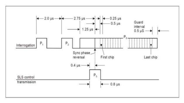
Figure 3-4. Mode S interrogation pulse sequence
