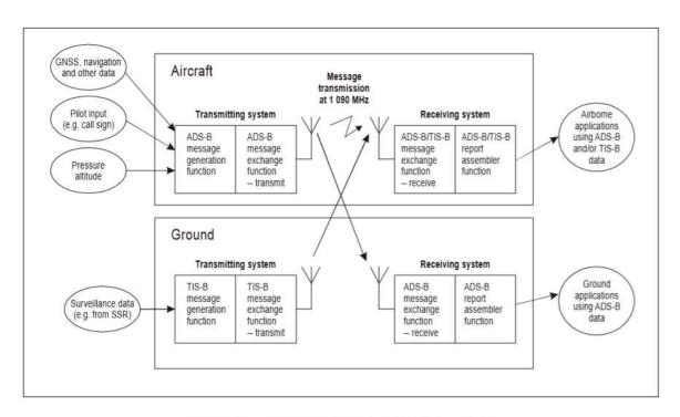
Figure 5-1. ADS-B/TIS-B system functional model
