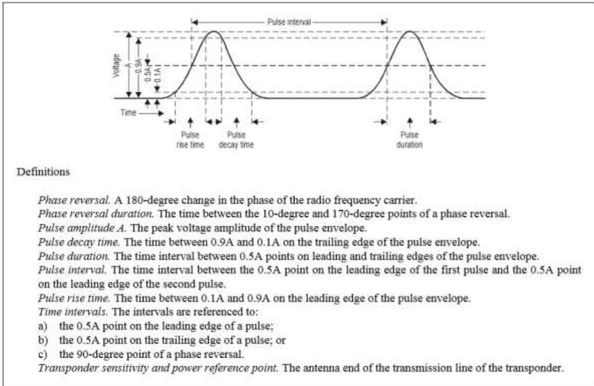
**Figure 3-1. Definitions of secondary surveillance radar waveform shapes, intervals and the reference point for sensitivity and power**
