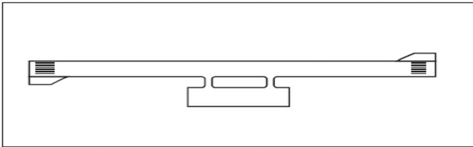
Figure 3-1. Typical turn pad layout
