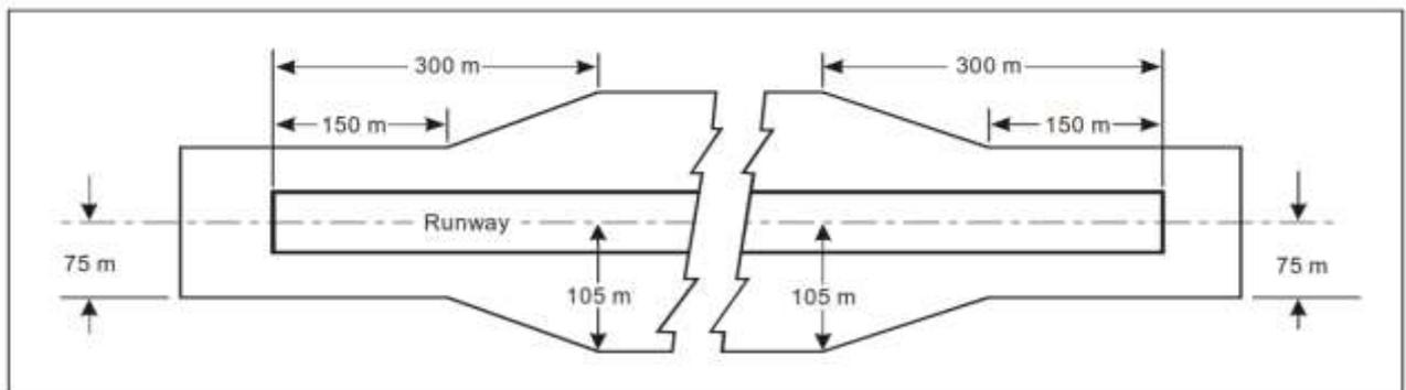
**Figure A-4. Graded portion of a strip including a precision approach runway where the code number is 3 or 4**
