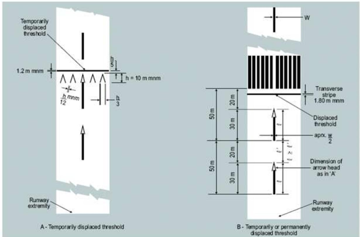
Figure 5-4. Displaced threshold markings
