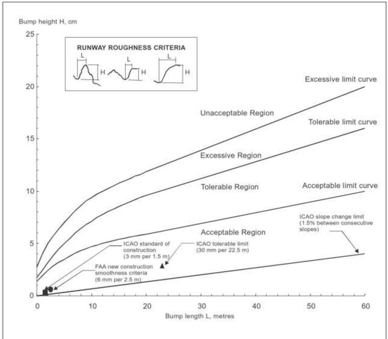
**Figure A-3. Comparison of roughness criteria**
