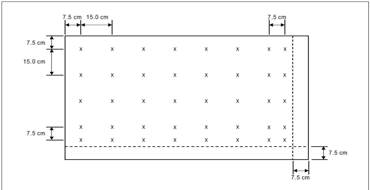
**Figure A4-1. Grid points for calculating average luminance of a sign**
