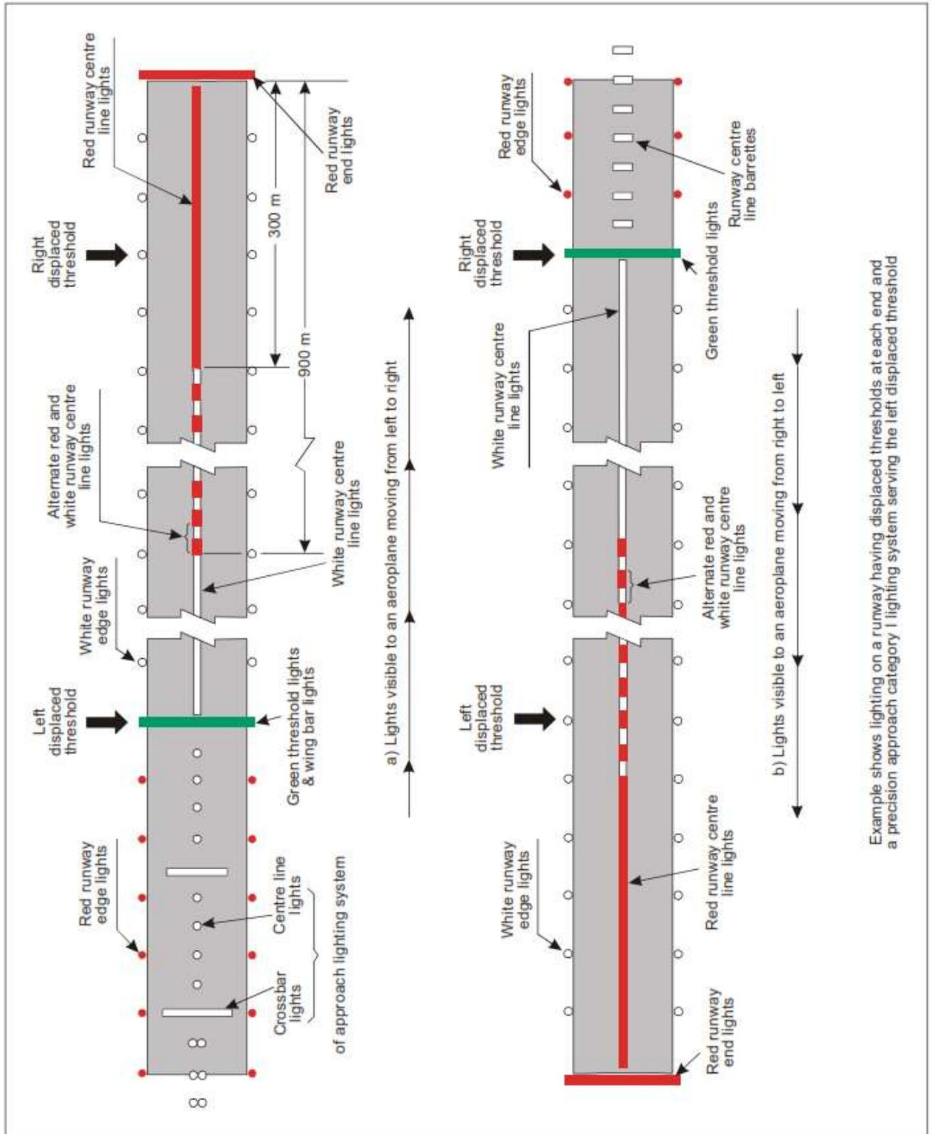
Example shows lighting on a runway having displaced thresholds at each end and a precision approach category I lighting system serving the left displaced threshold
