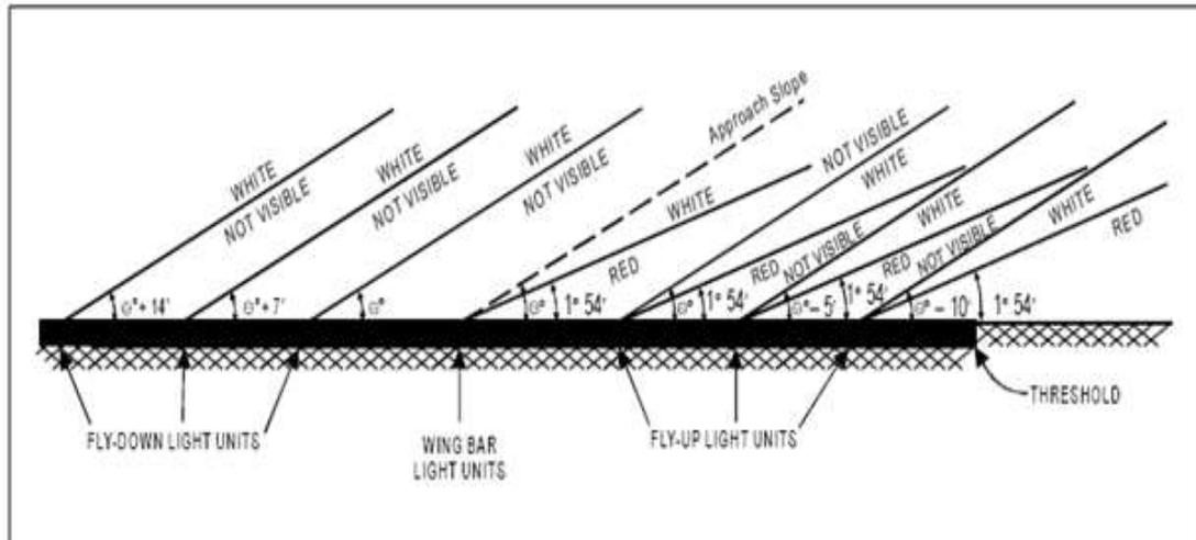
Figure 5-18. Light beams and elevation settings of T-VASIS and AT-VASIS
