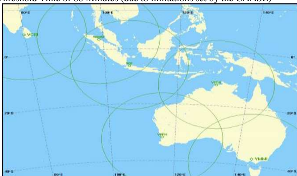
Example of Area of Operations for Aircraft that the Operations Specifications specified a Threshold Time of 90 Minutes (for Aircraft that satisfy the EDTO Capability to the CAASL)
