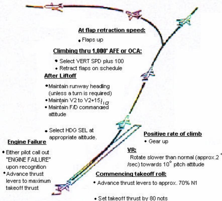
**Note: Above procedure and settings relevant to operators aircraft AOM**
