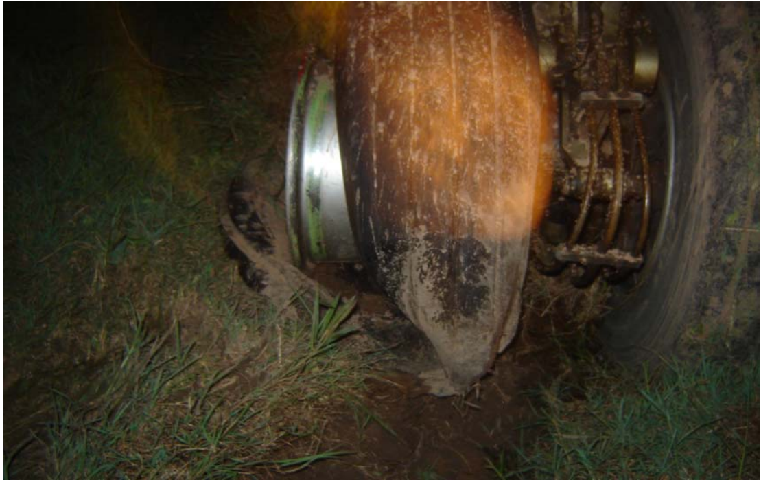
Aircraft right inboard tyre bust
