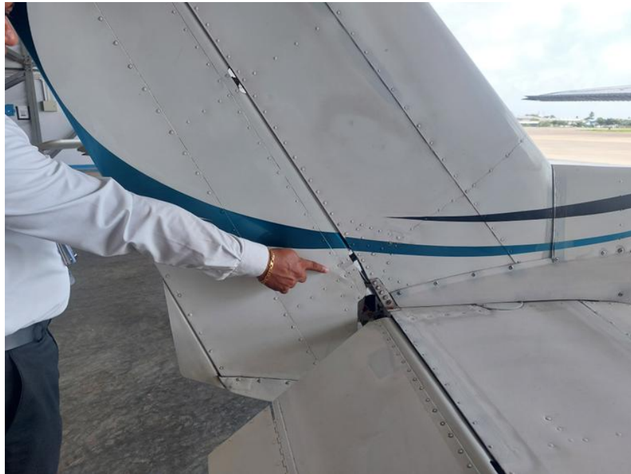
Figure 08: Wrinkles at the Rudder mounting Area
