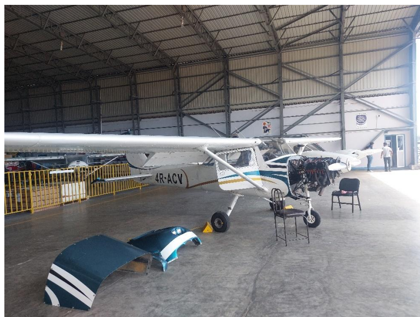
Figure 03: The effected Nose Landing Gear (bent backwards)
