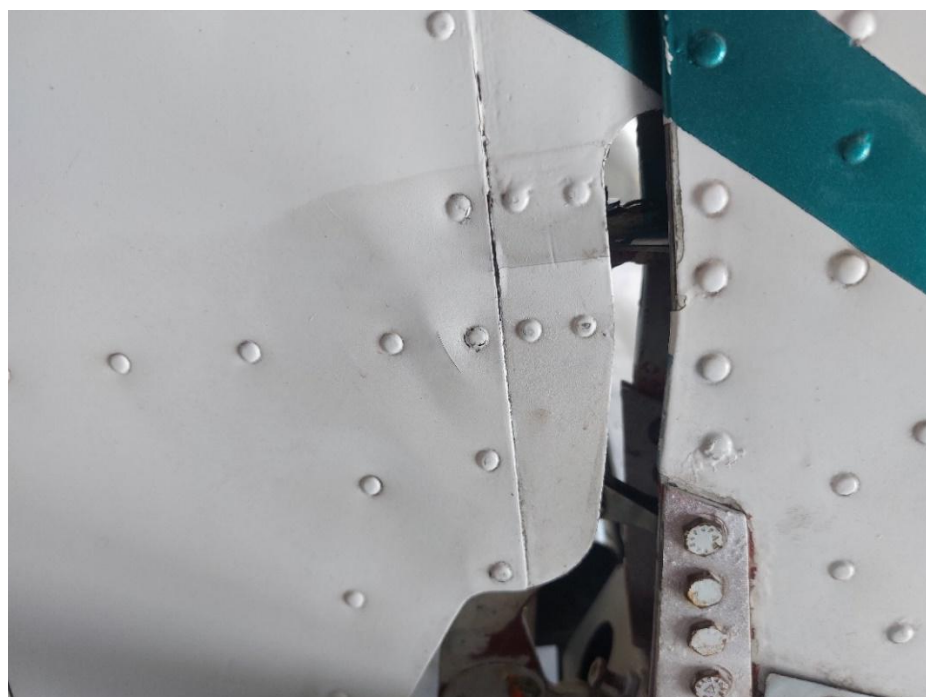
Figure 09: Wrinkles at the Rudder mounting Area
