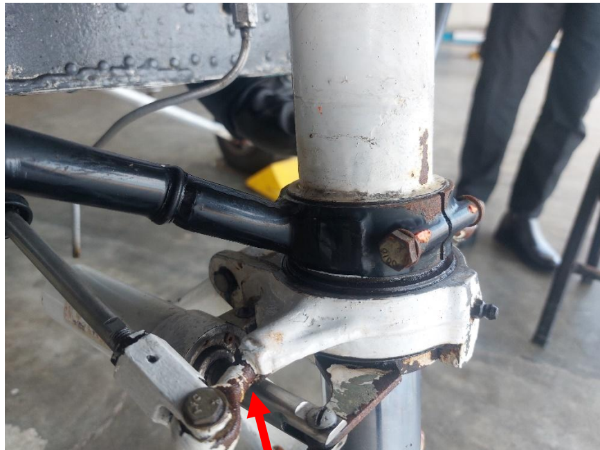
Figure 04: Distorted Torque Link
