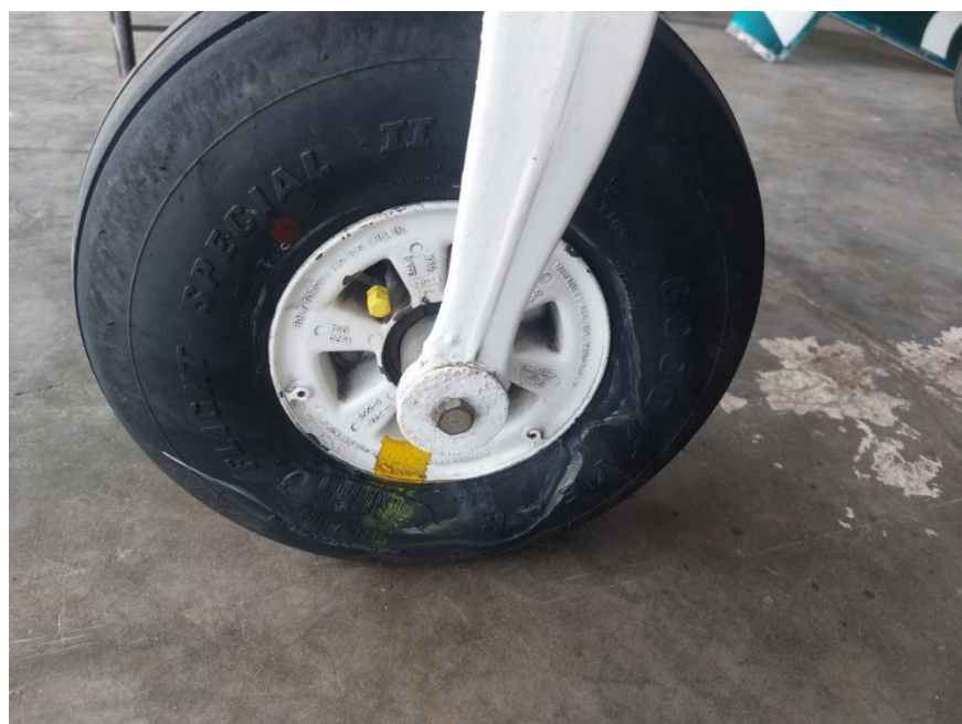
Figure 07: Impact Marks NLG
