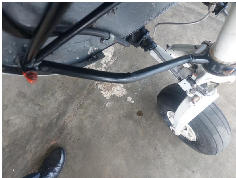
Figure 01: Damages sustained to the Engine mount
