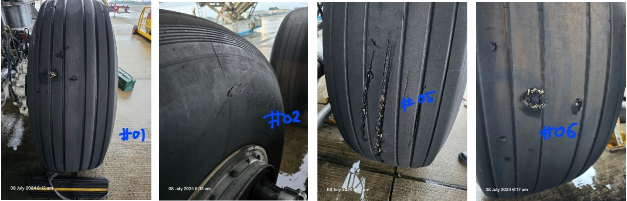
Figure 7 – Damages to the tyres of left MLG
